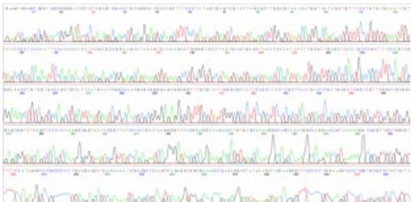
**Figure 17.** Taq FS dRhodamine dye terminator sequencing reactions with different amounts of ultrapure plasmid DNA purified using QIAGENtip 100. **A** 50 ng, **B** 200 ng, **C** 2.3 µg plasmid pTZ19R; primer: -21M13 primer. Note the different signal intensities in the header of each electropherogram.
